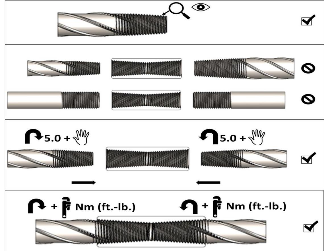
NOTE :Couplers must be assembled with calibrated torque wrench. Torque wrench must be calibrated at least every 24 months (+/- 15%).
